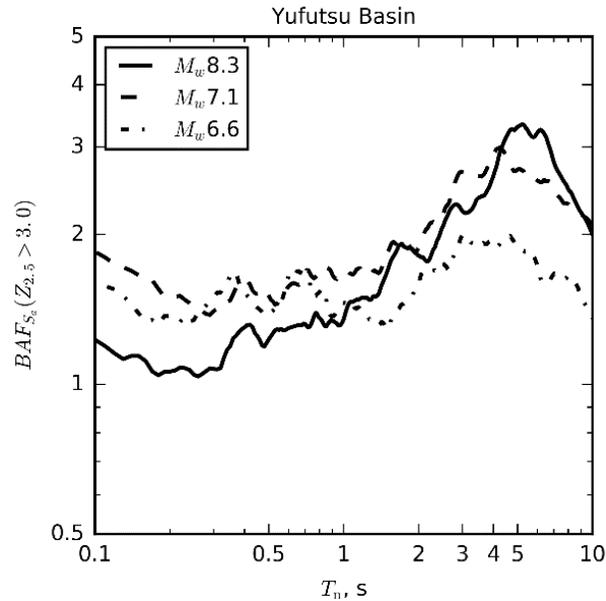
Figure 5.  $BAF_{Sa}$  with respect to the fundamental period of the structure for varying magnitude earthquakes.
