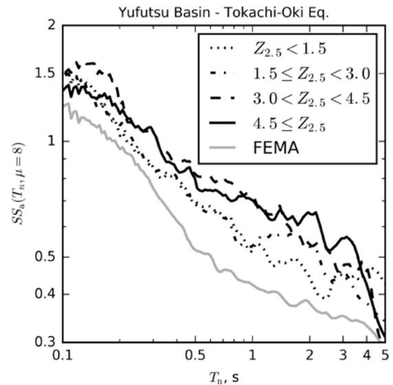
Figure 7. Median of  $SS_a$  with respect to the fundamental period of the structure for various  $Z_{2.5}$  bins
