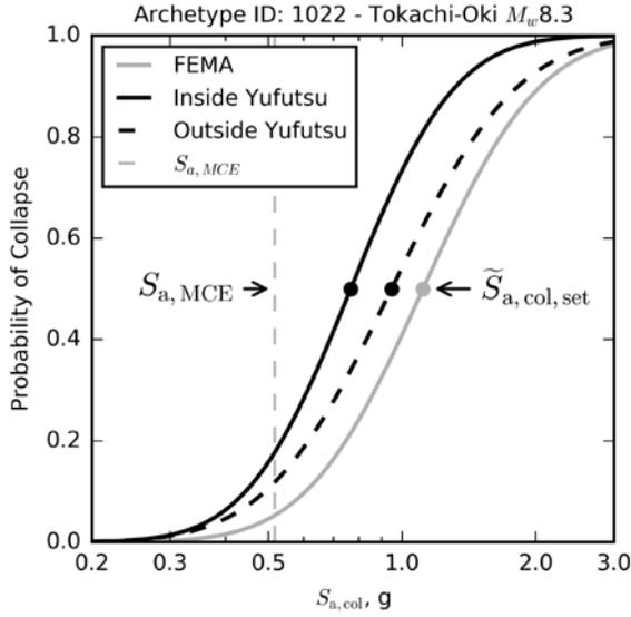
Figure 8. Collapse fragility functions for three ground-motion sets computed using spectral acceleration
