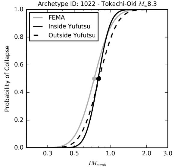
Figure 9. Collapse fragility functions for three ground-motion sets computed using  $IM_{comb}$
