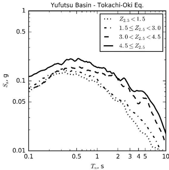
Figure 3. Median  $S_a$  with respect to the fundamental period of structure for recordings binned in terms of  $Z_{2.5}$  ranges.
