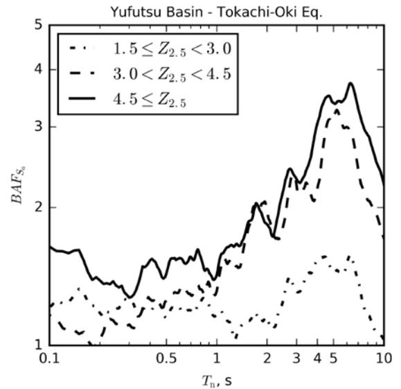
Figure 4. Basin Amplification Factors with respect to the fundamental period of structure for varying  $Z_{2.5}$  ranges.
