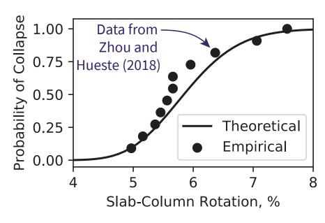
• The probability of collapse under an earthquake event can be computed using the equation below:
